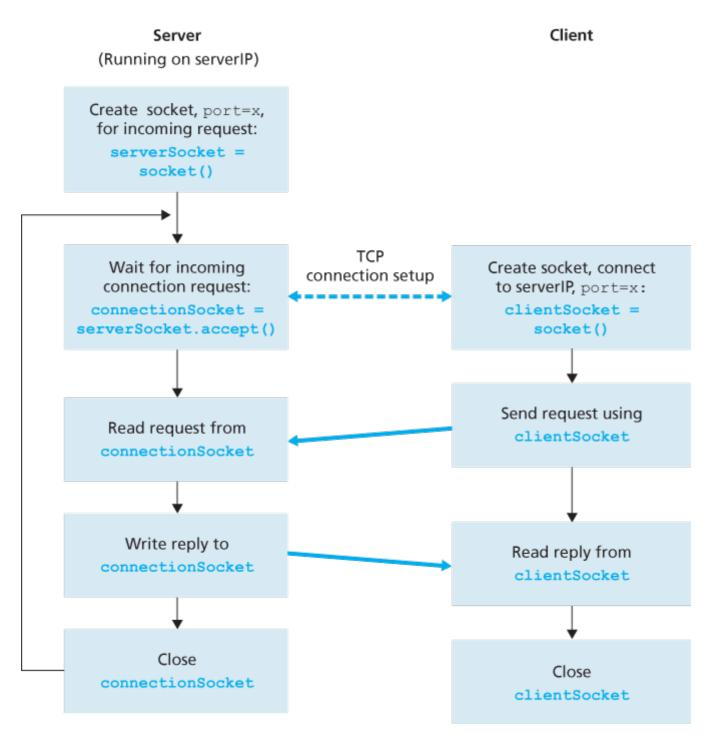
Figure 2.29 The client-server application using TCP
