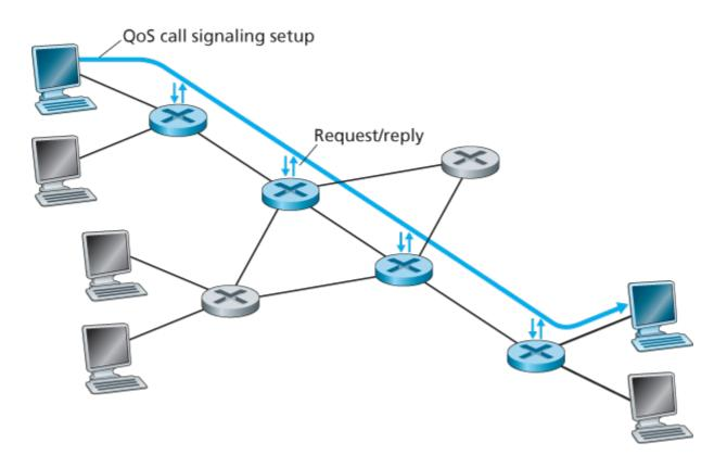
Figure 9.19 The call setup process
