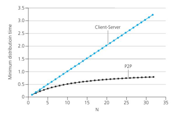
Figure 2.23 Distribution time for P2P and client-server architectures
