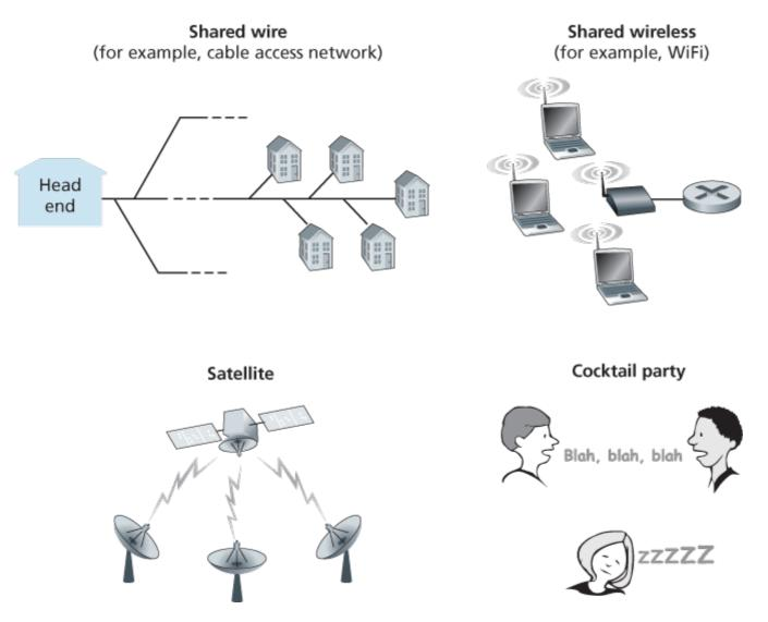
Figure 6.8 Various multiple access channels
