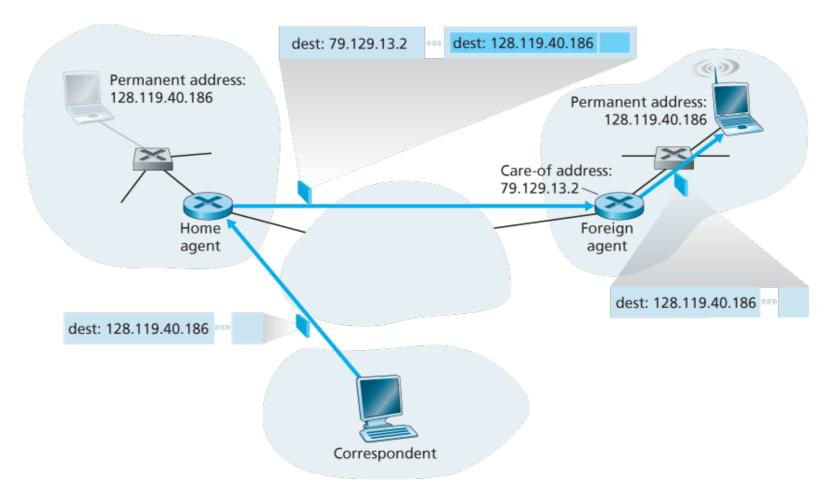
Figure 7.25 Encapsulation and decapsulation
