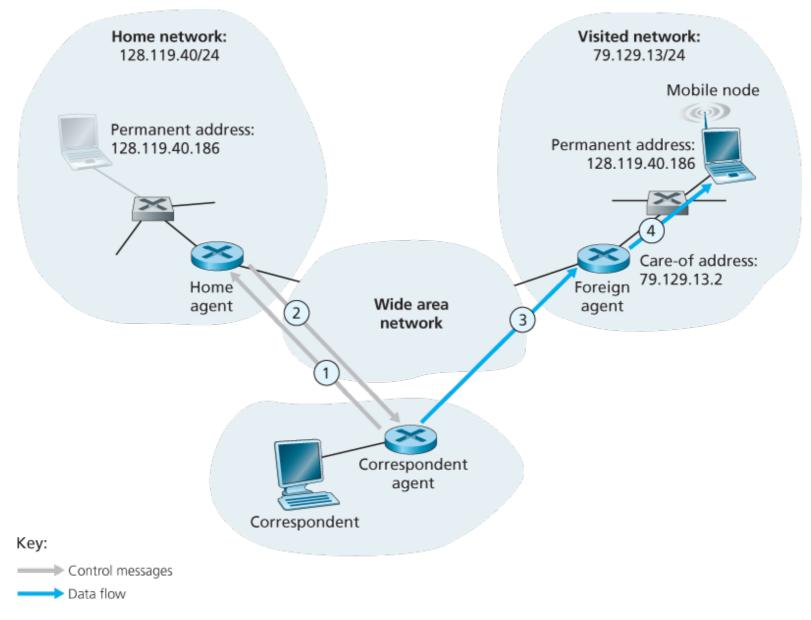
Figure 7.26 Direct routing to a mobile user
