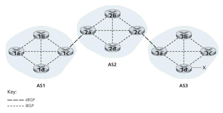
Figure 5.9 eBGP and iBGP connections
