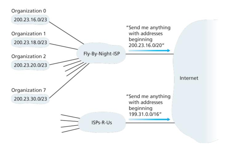
Figure 4.21 Hierarchical addressing and route aggregation
