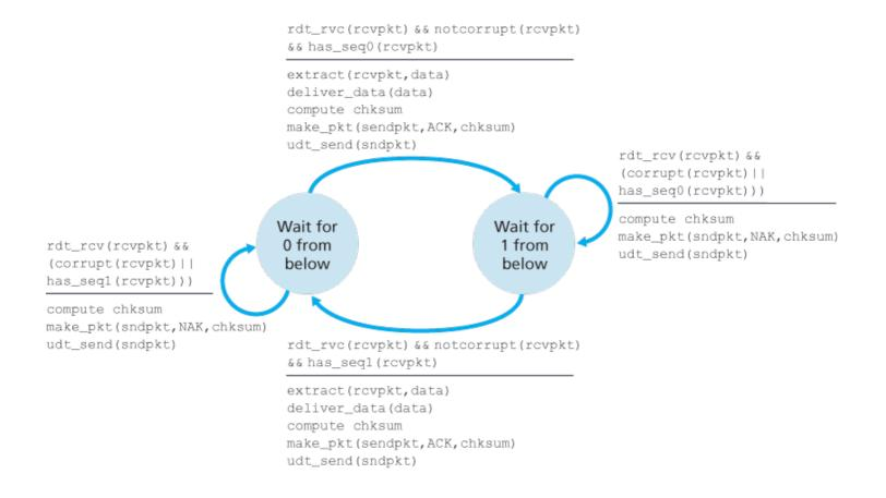
Figure 3.57 An incorrect receiver for protocol rdt 2.1
