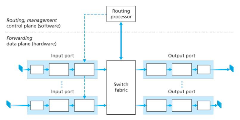
Figure 4.4 Router architecture
