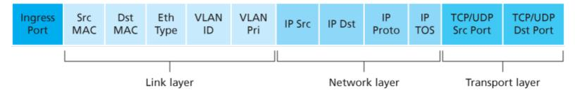
Figure 4.29 Packet matching fields, OpenFlow 1.0 flow table
