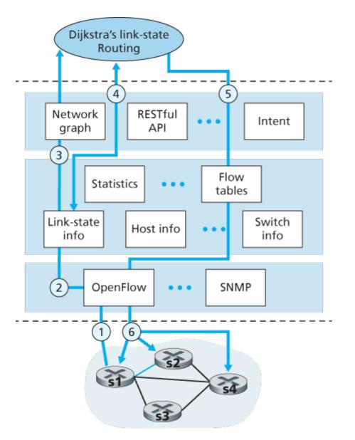
Figure 5.16 SDN controller scenario: Link-state change
