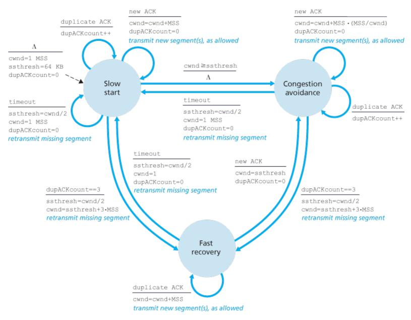
Figure 3.51 FSM description of TCP congestion control
