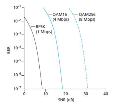
Figure 7.3 Bit error rate, transmission rate, and SNR
