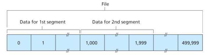
Figure 3.30 Dividing file data into TCP segments
