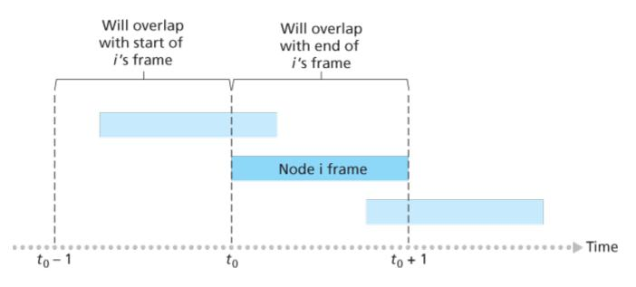
Figure 6.11 Interfering transmissions in pure ALOHA
