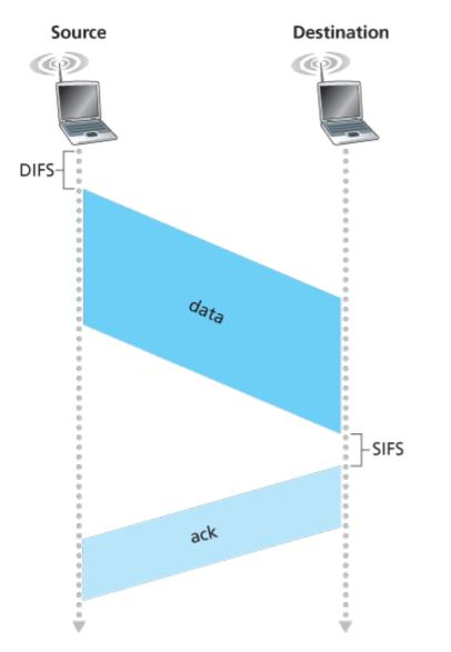
Figure 7.10 802.11 uses link-layer acknowledgments
