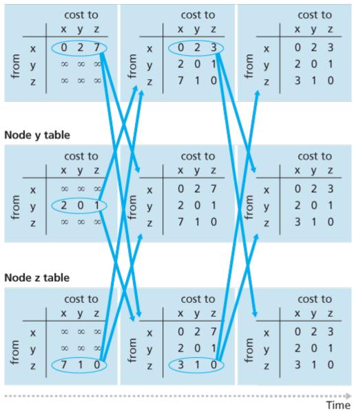
Figure 5.6 Distance-vector (DV) algorithm in operation
