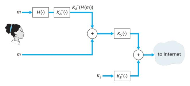
Figure 8.21 Alice uses symmetric key cyptography, public key cryptography, a hash function, and a digital signature to provide secrecy, sender authentication, and message integrity
