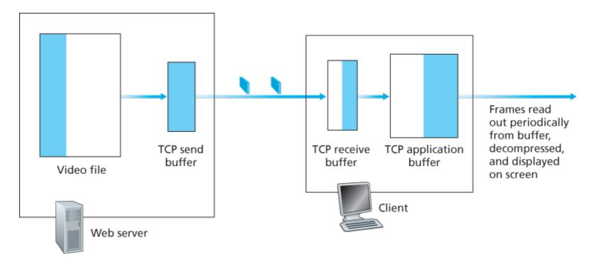
Figure 9.2 Streaming stored video over HTTP/TCP
