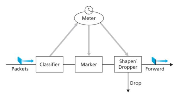
Figure 9.17 A simple Diffserv network example
