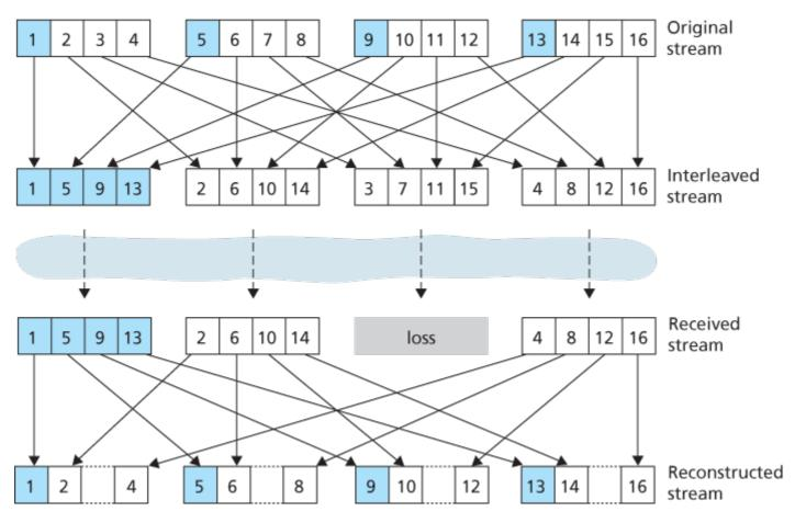
Figure 9.6 Sending interleaved audio
