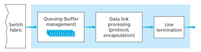
Figure 4.7 Output port processing
