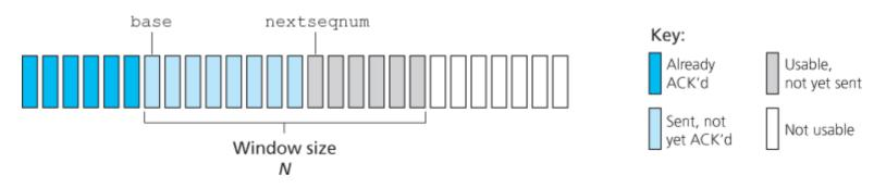
Figure 3.19 Sender's view of sequence numbers in Go-Back-N
