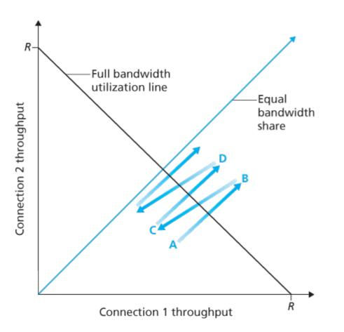
Figure 3.55 Throughput realized by TCP connections 1 and 2
