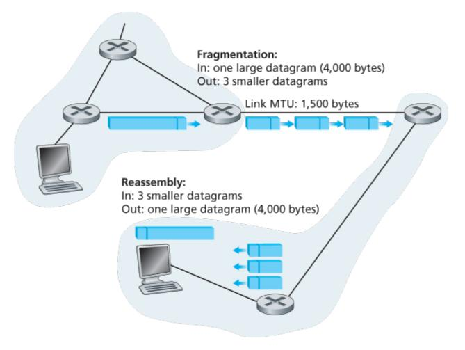
Figure 4.17 IP fragmentation and reassembly
