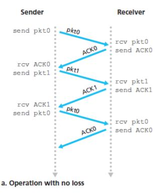
Figure 3.16 Operation of *rdt3.0*, the alternating-bit protocol
