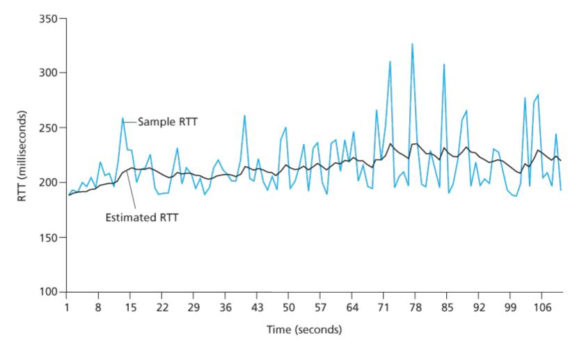
Figure 3.32 RTT samples and RTT estimates
