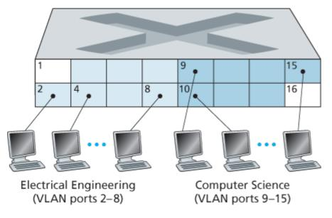
Figure 6.25 A single switch with two configured VLANs
