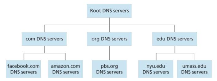
Figure 2.17 Portion of the hierarchy of DNS servers
