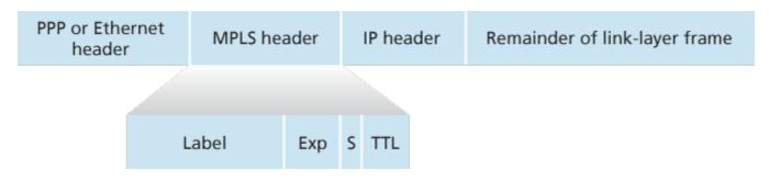
Figure 6.28 MPLS header: Located between link- and network-layer headers
