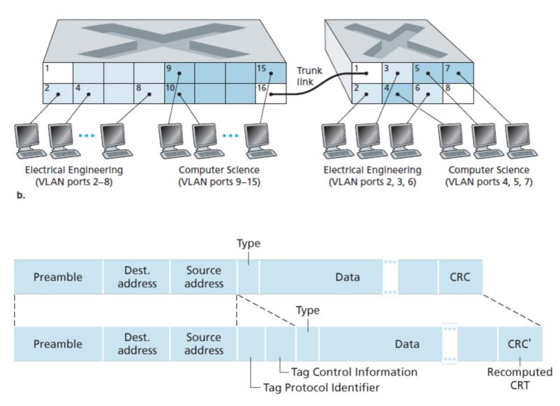
Figure 6.27 Original Ethernet frame (top), 802.1Q-tagged Ethernet VLAN frame (below)
