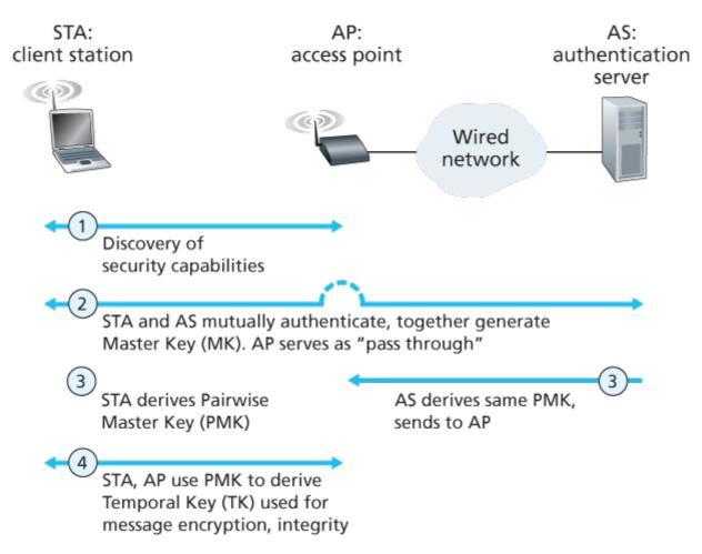
Figure 8.31 802.11i: Four phases of operation
