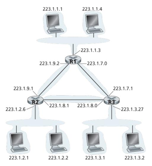
Figure 4.20 Three routers interconnecting six subnets
