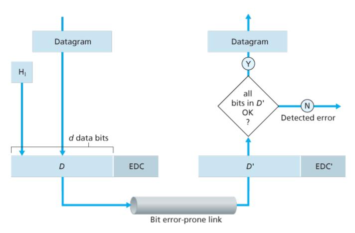
Figure 6.3 Error-detection and -correction scenario
