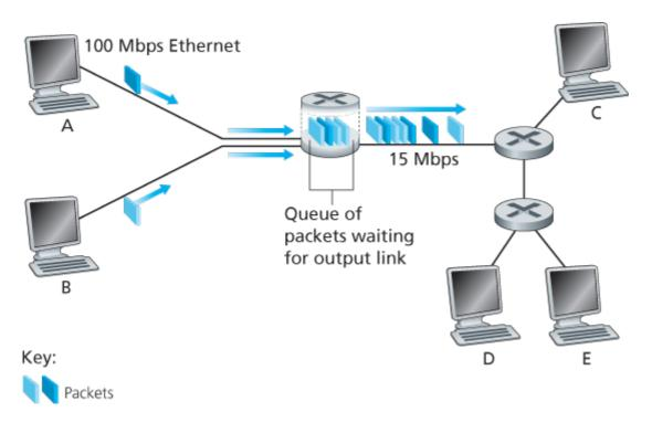
Figure 1.12 Packet switching
