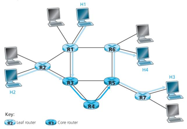
Figure 9.16 A simple Diffserv network example
