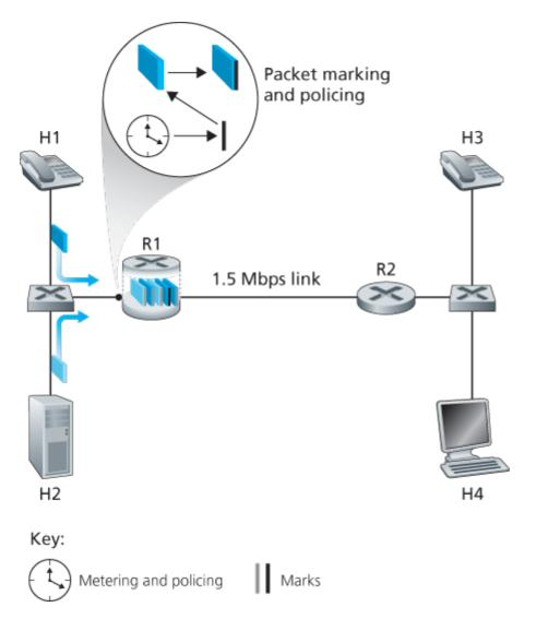
Figure 9.12 Policing (and marking) the audio and HTTP traffic classes
