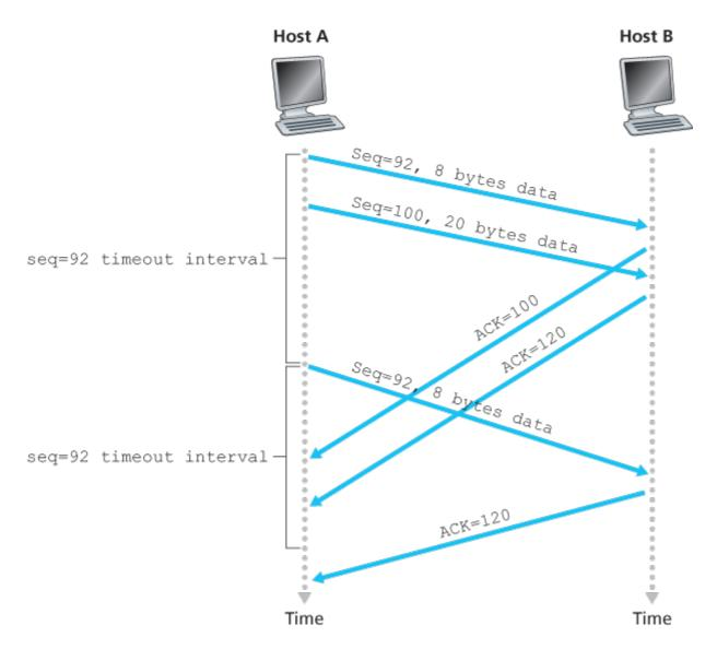
Figure 3.35 Segment 100 not retransmitted
