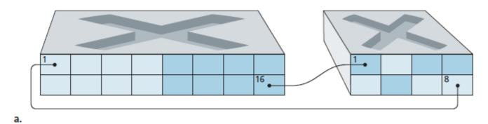
Figure 6.26 Connecting two VLAN switches with two VLANs: (a) two cables (b) trunked
