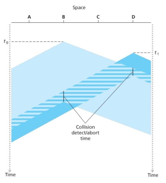
Figure 6.13 CSMA with collision detection
