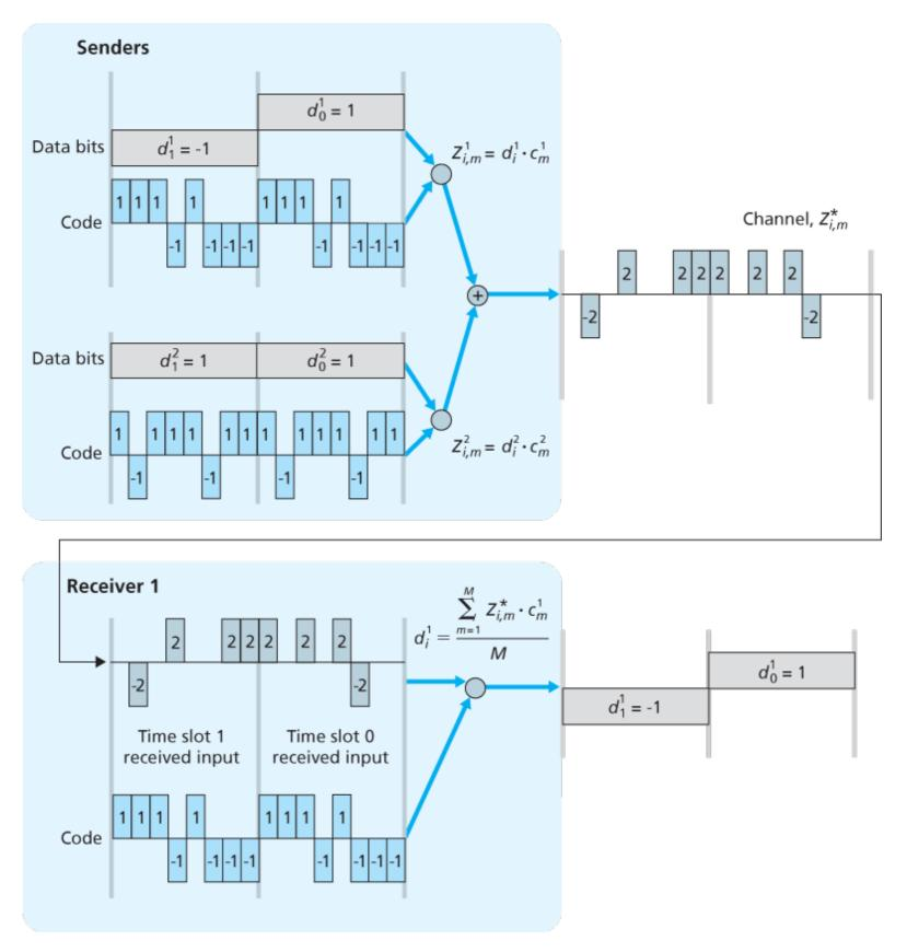
Figure 7.6 A two-sender CDMA example
