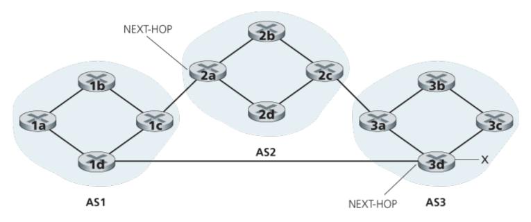
Figure 5.10 Network augmented with peering link between AS1 and AS3
