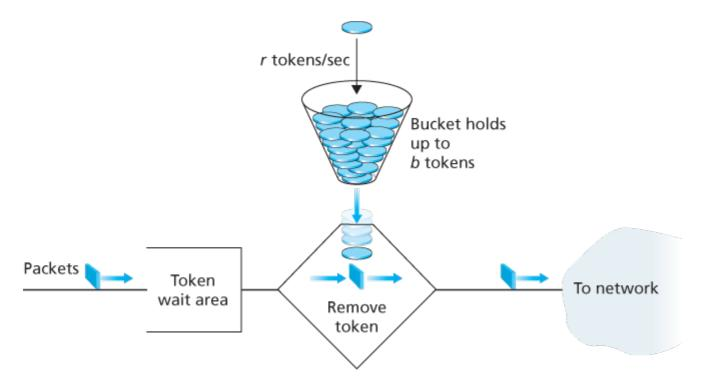
Figure 9.14 The leaky bucket policer
