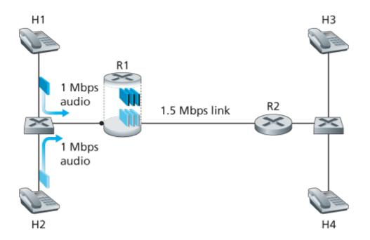
Figure 9.18 Two competing audio applications overloading the R1-to-R2 link
