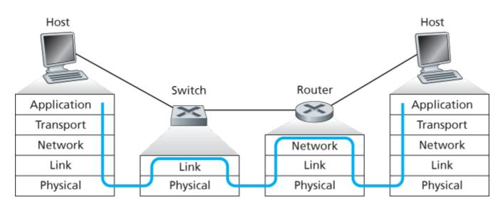
Figure 6.24 Packet processing in switches, routers, and hosts
