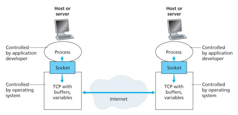
Figure 2.3 Application processes, sockets, and underlying transport protocol
