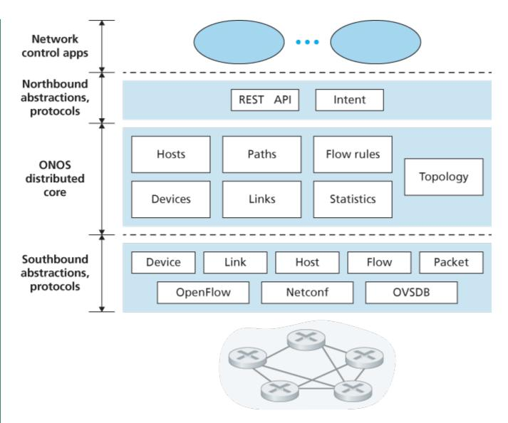
Figure 5.18 ONOS controller architecture
