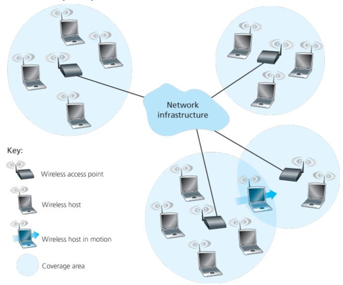
Figure 7.1 Elements of a wireless network
