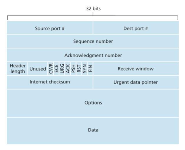
Figure 3.29 TCP segment structure
