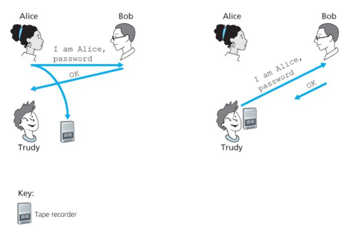
Figure 8.17 Protocol ap3.0 and a failure scenario
