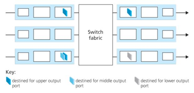
Figure 4.8 HOL blocking at and input-queued switch
