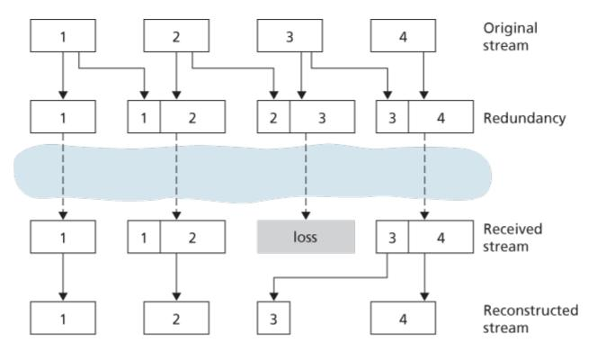
Figure 9.5 Piggybacking lower-quality redundant information
