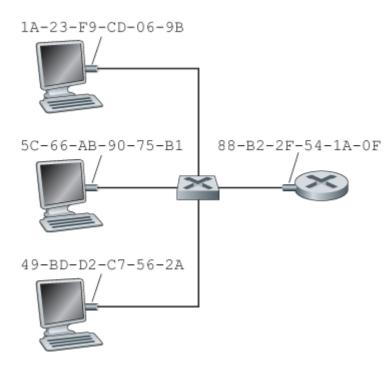
Figure 6.16 Each interface connected to a LAN has a unique MAC address
