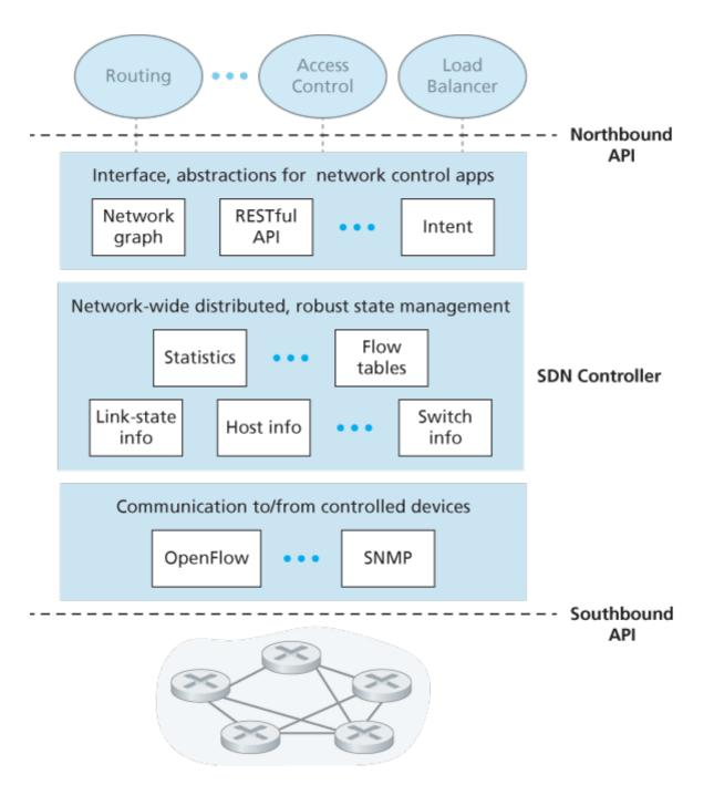
Figure 5.15 Components of an SDN controller
