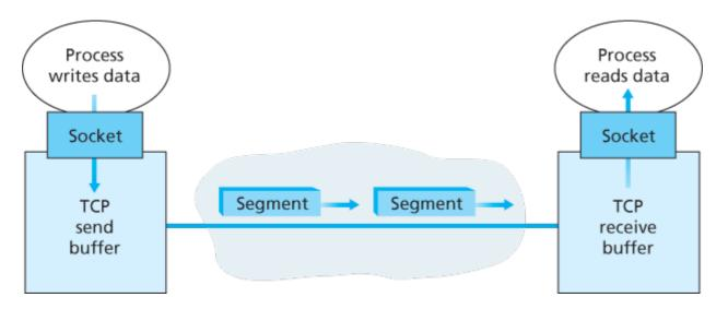
Figure 3.28 TCP send and receive buffers
