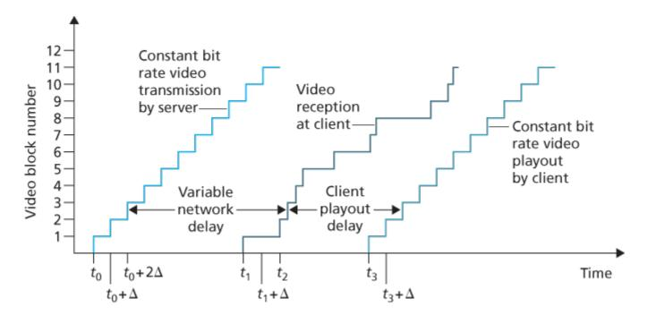
Figure 9.1 Client playout delay in video streaming
