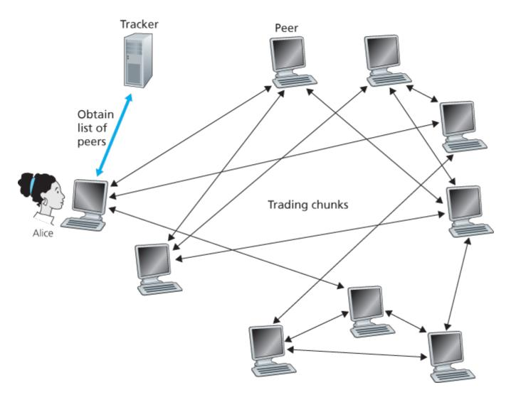
Figure 2.24 File distribution with BitTorrent
