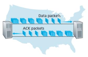
b. A pipelined protocol in operation
