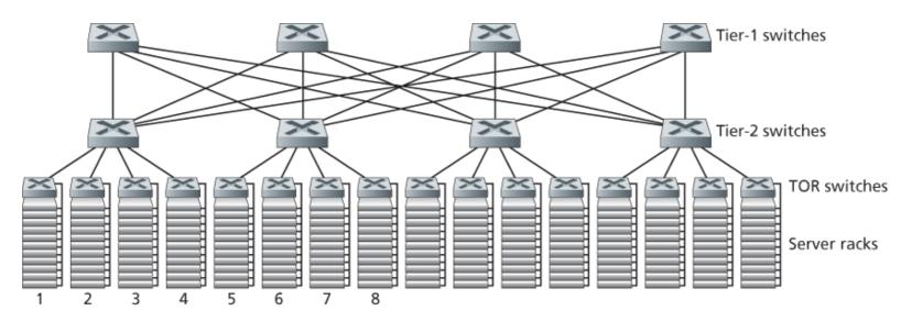
Figure 6.31 Highly interconnected data network topology
