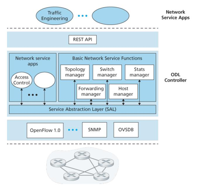
Figure 5.17 The OpenDaylight controller
