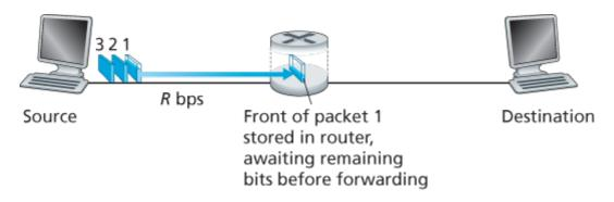
Figure 1.11 Store-and-forward packet switching
