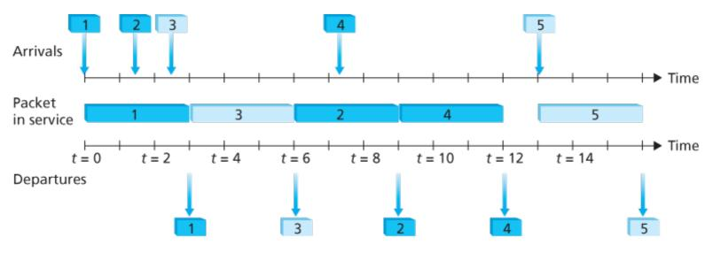
Figure 4.14 The two-class robin queue in operation
