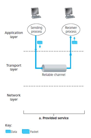
Figure 3.8 Reliable data transfer: Service model and service implementation
