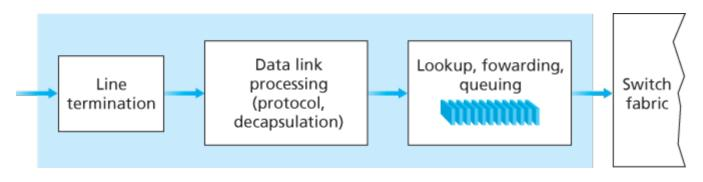
Figure 4.5 Input port processing
