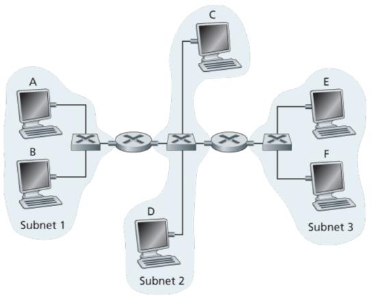
Figure 6.33 Three subnets, interconnected by routers
