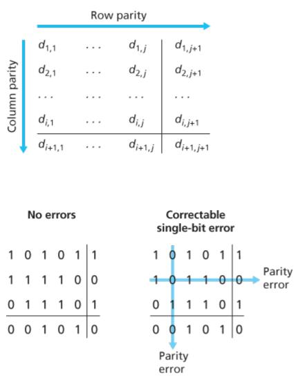
Figure 6.5 Two-dimensional even parity
