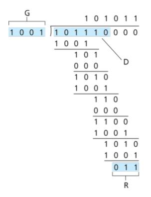
Figure 6.7 A sample CRC calculation
